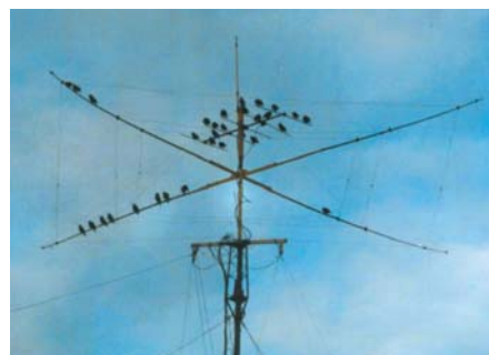
The three-band G6XN antenna by GM3SVE. The top mast section is aluminium scaffolding pole fixed to the top of a 40ft Tennamast via a rotator. The fibreglass rods are fixed to the mast using 2in aluminium angle.
